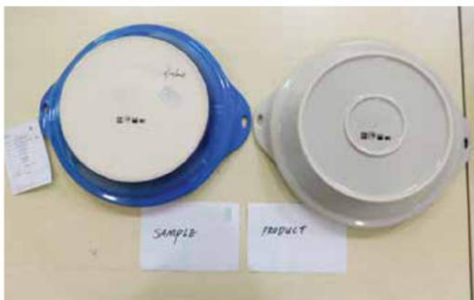
Figure 2. Comparing an approved sample to a mass-produced product.
